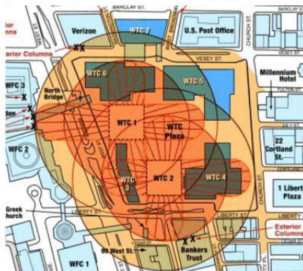
Figure 3. FEMA debris map for the Twin Towers
